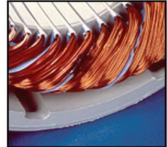
Winding Shorted Phase to Phase
