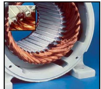
Winding Grounded at Edge of Slot
